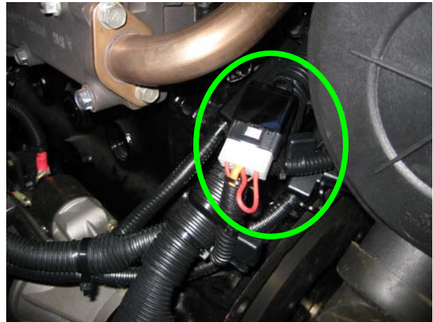
Correct Orientation Water can drain from connector
