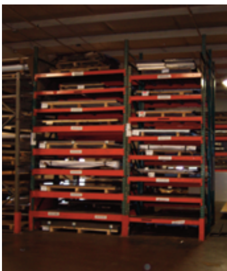
FIGURE 1 DeWys Manufacturing management determined that it could reduce the variety of material sheet sizes it bought, which will translate into tighter nests and less material waste. The newfound raw material storage space then can be turned into manufacturing space.
